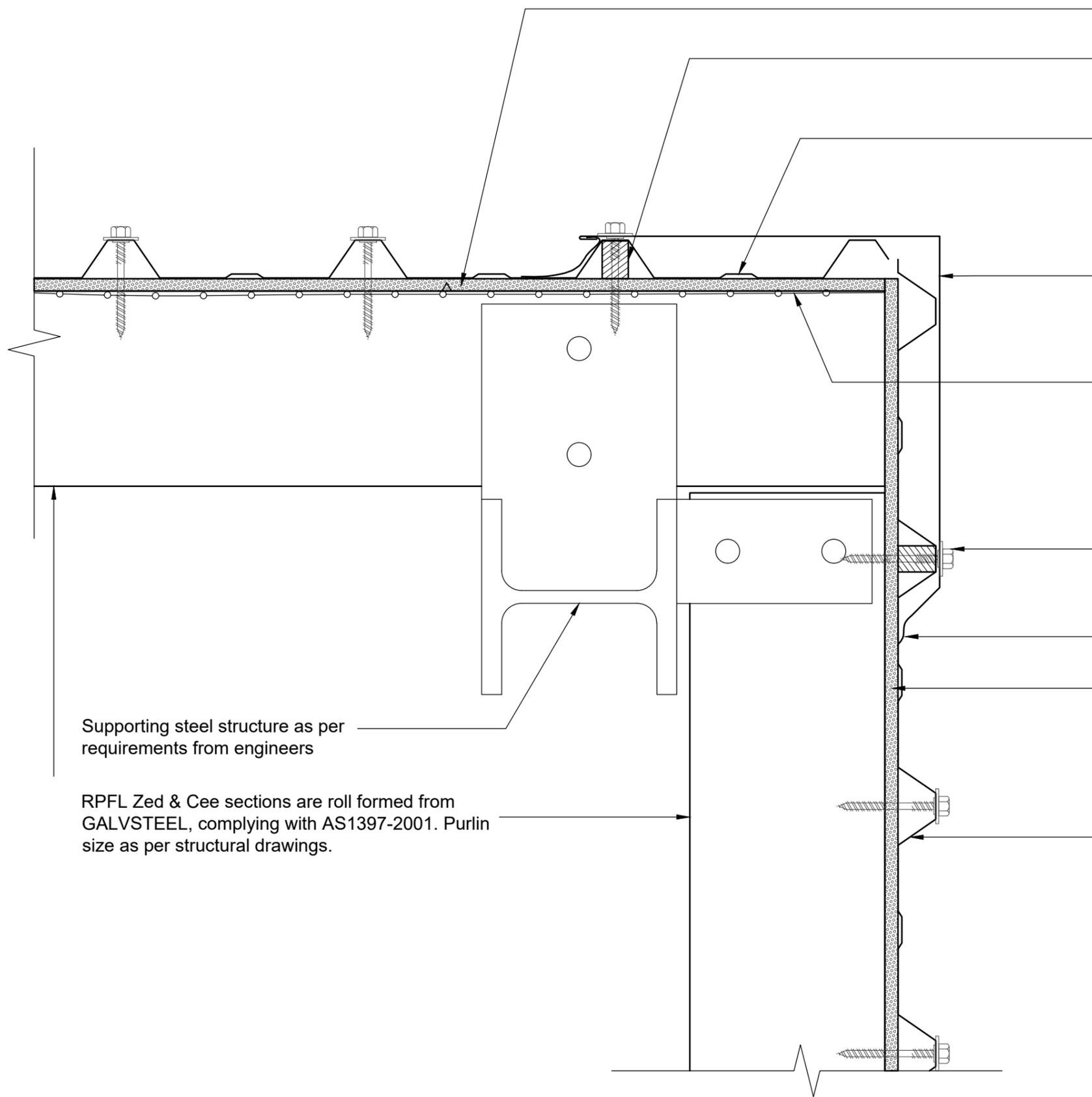
Kingspan AIR-CELL INSULINER Self-Supported 3-in-1 Insulation Vapour Barrier and Radiant Barrier or 430 WF Med. duty sisalation
