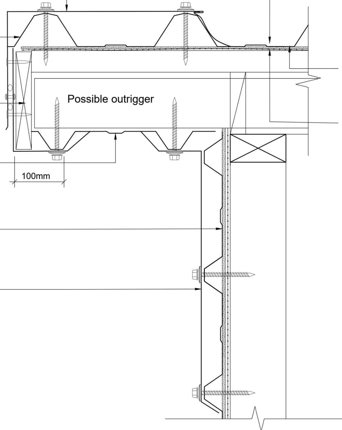
Flashguard Soft Edge flashing for metal roof accessories
