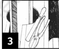
3 Cut out marked portions of roof, filing away sharp edges and install pipe securely in place. Where required, support cut sections of sheet with additional framing.
