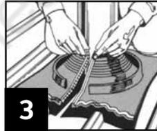
3 With clip in down-stream position tension top of cone around pipe and engage metal teeth in opposing pockets.
