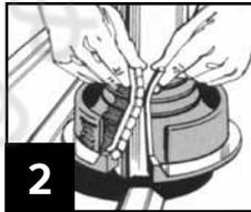
With clip in down-stream position, tension top of cone around pipe and engage metal teeth in opposing pockets.
