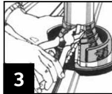
To assist in locating clip into pocket, place hand behind the seam. Fasten clip with pliers or multi-grips, working from top to base. **Do not overcrimp.**
